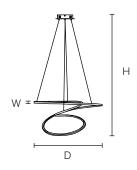
**AD-NA-1607A-8B:** W 23.5mm x D Ø800mm x H 1500mm (W 0.93" x D Ø31.5" x H 59.06")
